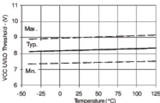
Figure 21B. V<sub>CC</sub> Undervoltage Threshold(-) vs Temperature
