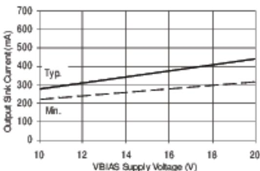
Figure 23B. Output Sink Current
