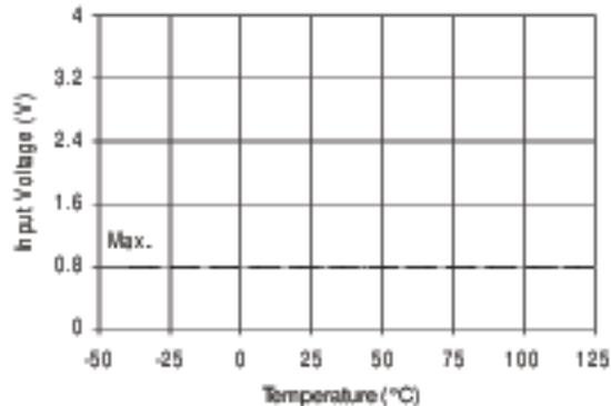
Figure 13A. Logic "0" Input Voltage (IR2101)
