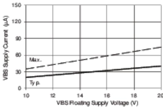
**Figure 17B. V<sub>BS</sub> Supply Current vs Voltage**
