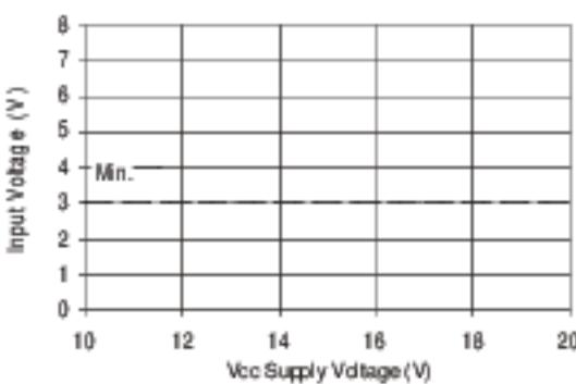
Figure 12B. Logic "1" Input Voltage (IR2101)
