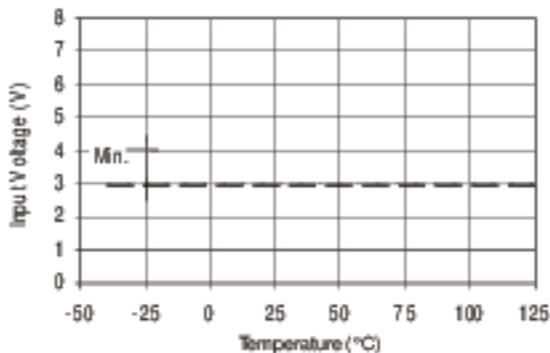
Figure 12A. Logic "1" Input Voltage (IR2101)
