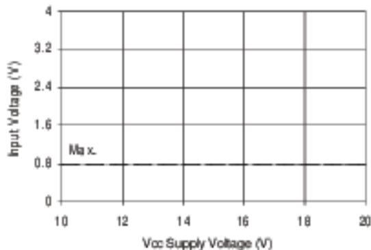
Figure 13B. Logic "0" Input Voltage (IR2101)
