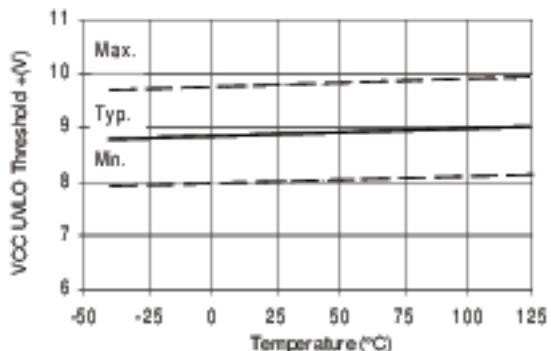
Figure 21A. V<sub>CC</sub> Undervoltage Threshold(+) vs Temperature
