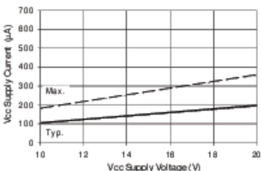
**Figure 18B. V<sub>CC</sub> Supply Current vs Voltage**
