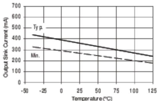
Figure 23A. Output Sink Current
