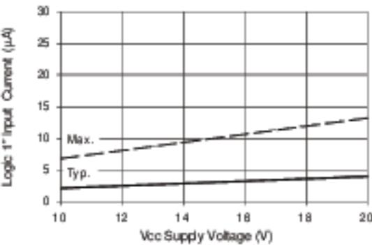
**Figure 19B. Logic "1" Input Current vs Voltage**
