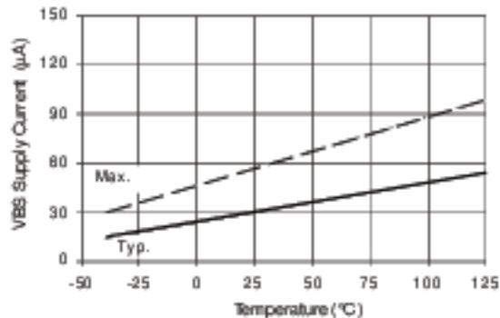
**Figure 17A. V<sub>BS</sub> Supply Current vs Temperature**
